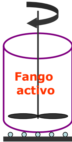
Sequential batch reactor
